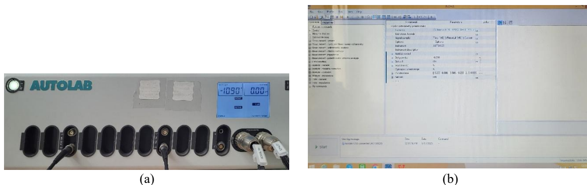
Fig. 1.2. AUTOLAB 302N potentiostat (a) and NOVA interface (a) used for conducting electrochemical experiments
